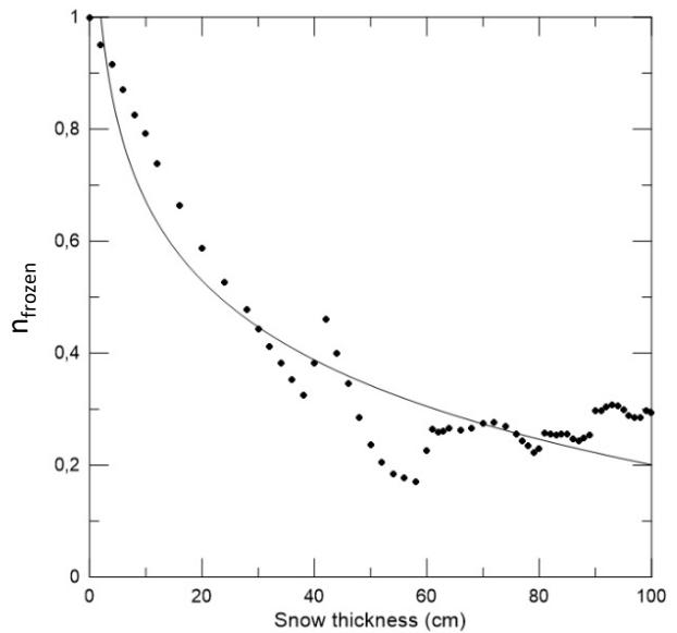
$$n_{\text{frozen}} = T_{\text{surface}} / T_{\text{air}}$$
